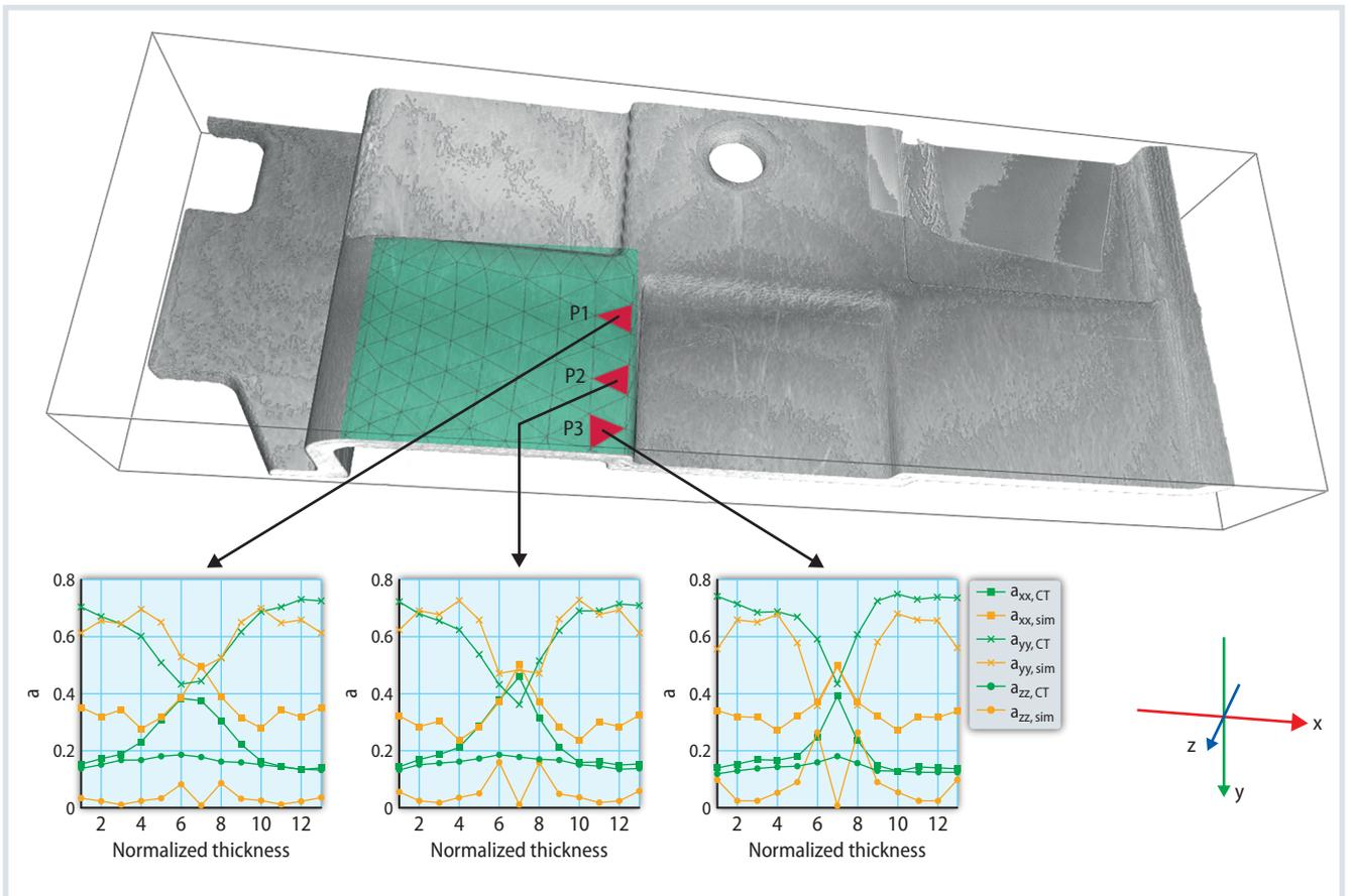
**Fig. 3.** Diagonal components of the 2nd order orientation tensor, comparison of the orientation predicted by injection molding simulation (orange) and the orientation measured in the 3D images with highest resolution (green). The position of the regions used in the simulation is marked red in the volume rendering source: ITWM, graphic: © Hanser
