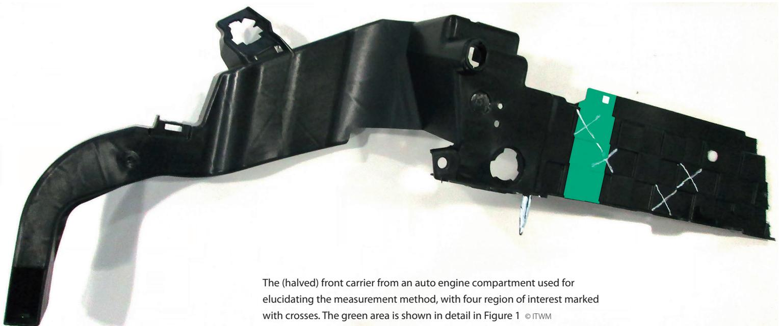
The (halved) front carrier from an auto engine compartment used for elucidating the measurement method, with four region of interest marked with crosses. The green area is shown in detail in Figure 1 © ITWM
