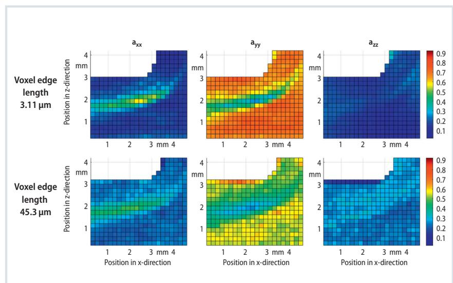
**Fig. 2.** Diagonal components of the 2nd order orientation tensor measured from the CT images.
